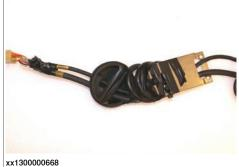
Run the cable harness through the cable guide and then into and through the upper arm tube.
